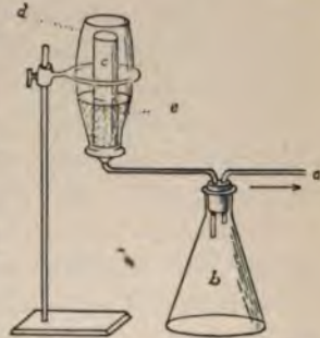
FIG. 40. — Chamberland's bougie arranged with lamp funnel for filtering a small quantity of fluid.
